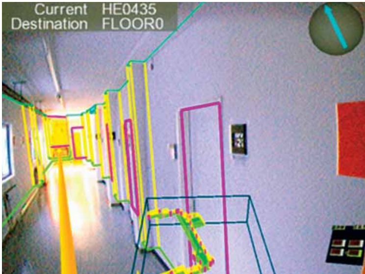
7 Indoor Signpost: the overlay shows a world in miniature and an arrow points to the suggested exit highlighted in yellow.
