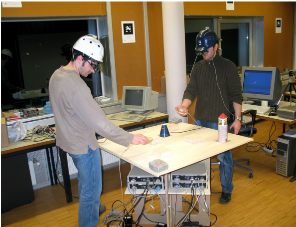
Figure 4. Dual-user setup using a magnetic tracker
